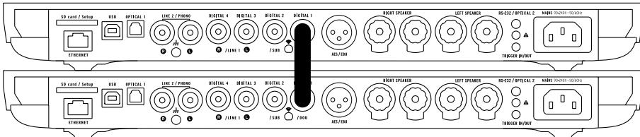
To set up your system in Dual-Mono, connect each loudspeaker to one Expert Pro and connect them with a digital cable (S/PDIF or S/PDIF-AES/EBU).
