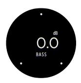
Low frequencies adjustment from -18dB cut to +18dB boost using a low-shelf filter structure.
