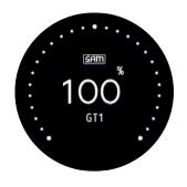
If a SAM profile is loaded, Low frequency extension: 0%: speaker natural bandwidth 100%: speaker bandwidth augmented thanks to SAM (by default)
