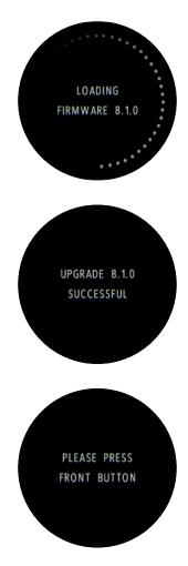
The upgrade should start automatically without pressing any button. When the upgrading process is complete, the display will indicate «Upgrade successful, please press front button » Your Devialet will be operable with the latest firmware and ready to play music.
