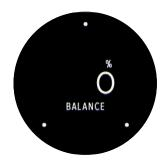
Left/Right Balance adjustment from -100% (full stereo incoming content sent to left channel only) to +100% (full stereo incoming content sent to right channel only). Setting is made remixing stereo incoming content into mono (by default) to perform music independent adjustment. 0% setting bypasses this stage.
