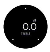
High frequencies adjustment from -18dB cut to +18dB boost using a high-shelf filter structure.
